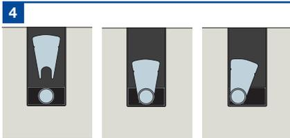
After a predetermined time period (generally 90-120 days), when movement between the slabs has stabilised and the joint between the slabs has been filled, the dowel is ready to be locked.
