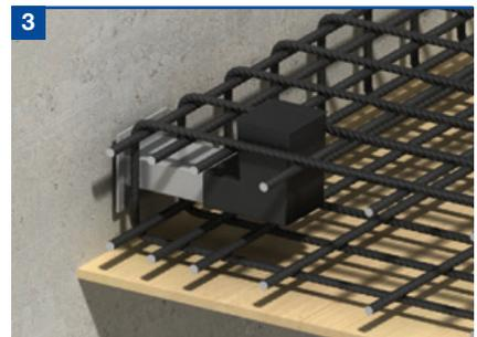
Puncture the label of the sleeve to reveal the cylindrical sleeve only. Push the sleeve over the dowel until it is flush with the concrete. Tie sleeve to reinforcement and pour concrete.
