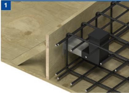
Nail the sleeve to the formwork either central in the slab or for slab depths over 300mm so the top of the void former is level with the top of the slab. Do not remove the label over the nailing plate as this prevents ingress of concrete into the sleeve. Fix the local reinforcement, as specified on engineer's drawings.
