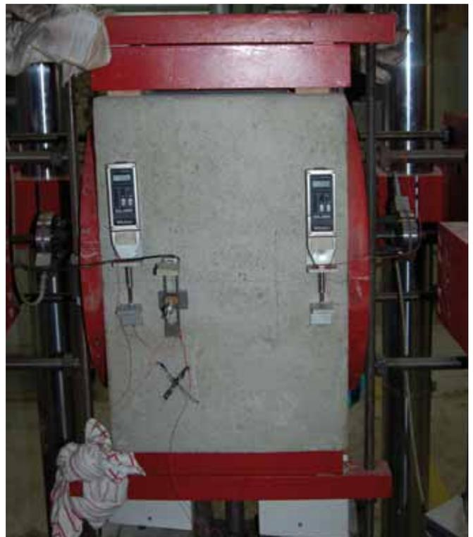
Test setup for cyclic load test
