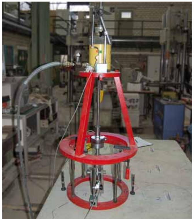
Test setup; pull-out test
