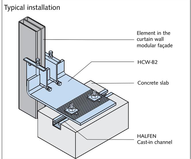
HALFEN Brackets HCW-B2 are made in grade S355 quality galvanized steel. The vertical adjustability is  $\pm 24$  mm. Three dimensional adjustability is ensured when used in combination with HALFEN Cast-in channels HTA-CE.
