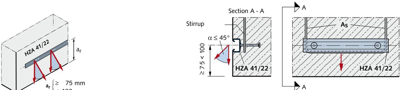
Figure 2: additional reinforcement placement
