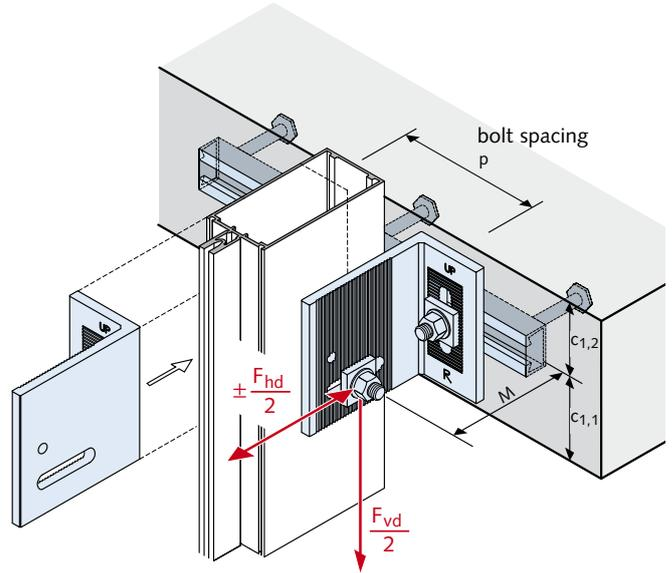
To guarantee correct installation, the HCW-ED brackets are marked 'R' for right, 'L' for left and 'UP' for top.
