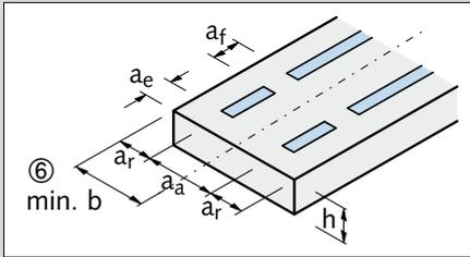
① If the (trapezoidal sheet metal) channels are placed so that the anchors of adjacent channels are offset by at least 200 mm, the axial spacing  $a_a$  may be reduced to 80 mm.
