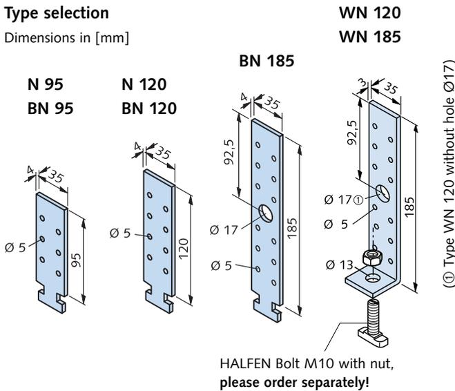
To provide an optimal base for roof framework, continuous HTA-CE HALFEN Cast-in channels or HTA-CE HALFEN Cast-in channels short elements can be used in concrete, reinforced concrete ring beams or slabs. The type of HTA-CE HALFEN Cast-in channels, nailing straps and nails depend on the assumed loads (e.g., wind force)
