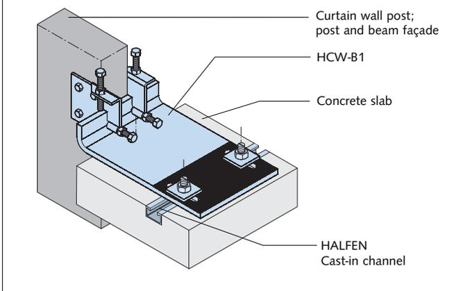
HALFEN Brackets HCW-B1; for installing to the top of concrete slabs, are available in two load ranges and three cantilever sizes. The brackets are made in grade S355 quality galvanized steel. Vertical adjustability is  $\pm 10$  mm. Three dimensional adjustability is ensured when used in combination with HALFEN HTA-CE Cast-in channels.
