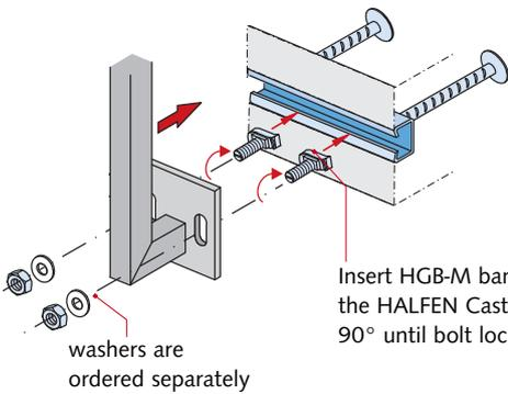
Insert HGB-M banister bolts into the HALFEN Cast-in channel (turn 90° until bolt locks in place).
