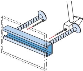
Where possible, use stainless steel nails to avoid corrosion.
