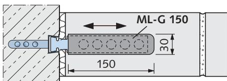
Permits movement in the longitudinal anchor direction, e.g. in long masonry bonds or partition walls adjoining concrete load bearing structures; prevents cracks forming.
