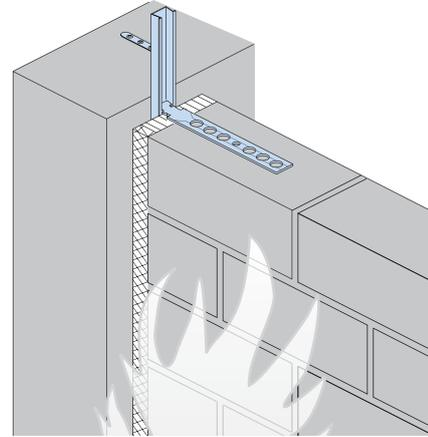
Connection of a load bearing solid wall as a firewall according to DIN 4102 T4 Paragraph 4.8.4 (figure 20.2)
