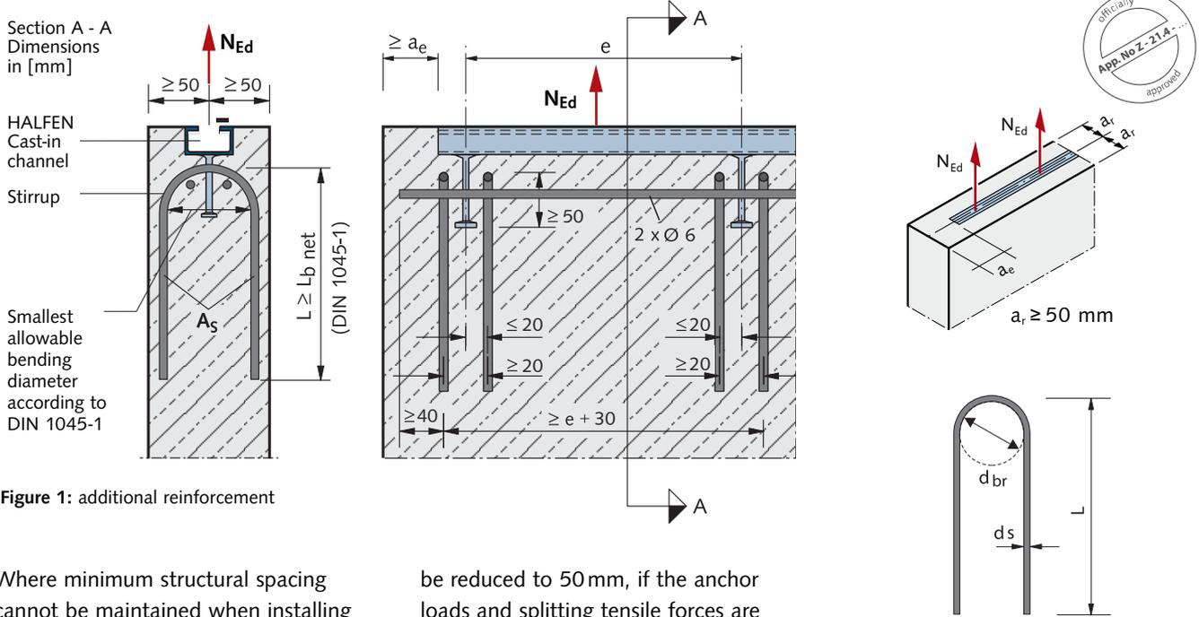
Figure 1: additional reinforcement
