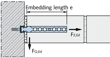
Plan view; facing brickwork attachment
