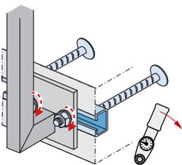
Tighten the nuts using a torque wrench. See table on the right for torque values
