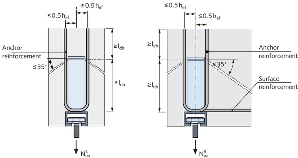
For conditions where the factored tensile and shear force exceed the concrete breakout strength of the HALFEN Anchor Channel or where the breakout strength is not evaluated, it is permitted within AC232 that the nominal strength can be that of anchor reinforcement properly placed as shown in the figures to the left.
