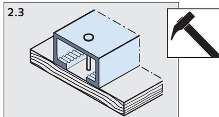
2.3 Fix to timber formwork with nails through the pre-punched holes in the back of the channel.
