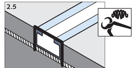
2.5 Fixing directly to the reinforcement: Attach the HALFEN Anchor Channel with reinforcement tie-wire.
