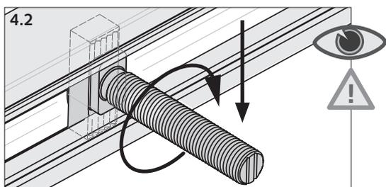
4.2 Insert the HALFEN T-bolt into the channel slot. After a 90° turn clockwise the HALFEN T-bolt locks into position. (Check whether the notch is perpendicular to the longitudinal channel axis)
