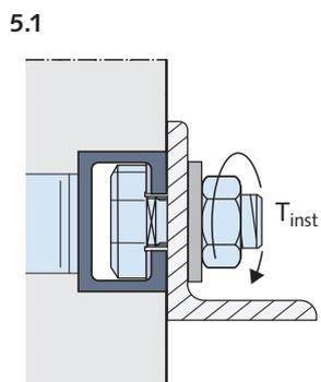
Tighten the nut with the installation torque  $T_{inst}$ . Exceeding the given installation torque  $T_{inst}$  according to this
