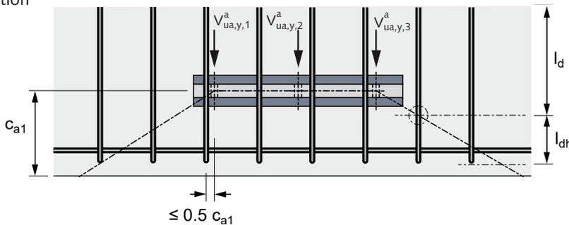
The anchor reinforcement of an anchor channel shall be designed for the highest anchor load,  $V_{ua,y}^a$  ( $V_{ua,x}^a$ ) of all anchor but at least for the highest individual load,  $V_{ua,y}^b$  ( $V_{ua,x}^b$ ) acting on the channel.
