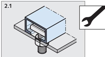
2.1 Secure with a HALFEN T-bolt through the formwork.
