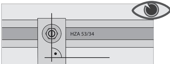
6. After tightening the nut, check whether the T-bolt is properly installed. If the notch is not perpendicular to the longitudinal channel axis, the T-bolt must be completely loosened, re-aligned, re-tightened; finally re-check the orientation of the notch is now correct.
