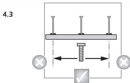
4.3 Alignment of the HALFEN T-bolt: It is not allowed to install HALFEN T-bolts beyond the center line of the end anchors.
