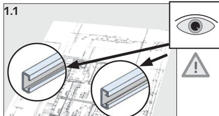
1.1 Select the HALFEN Anchor Channel according to the design plans.
