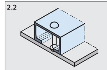
2.2 Using rivets or screws (supplied by the contractor) through the pre-punched nail holes in the HALFEN Anchor Channel.
