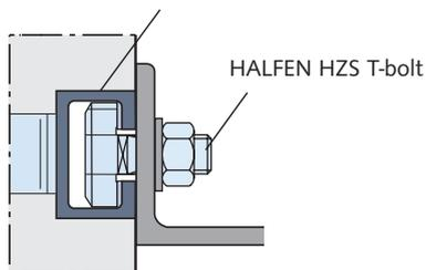
HALFEN Anchor Channels and T-bolts are available in a wide range of profile sizes/diameters and lengths allowing them to be utilised for a wide variety of applications in construction and industrial projects. The system is available in hot-dip galvanised and stainless steel to ensure long lasting performance. Engineered to the highest American standards, HALFEN HZA Anchor Channel system is a proven safe, simple and cost effective method of anchorage to concrete.
