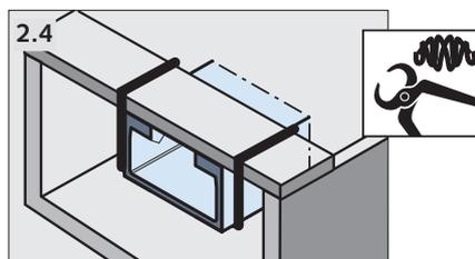
2.4 With a fixing bracket: Meticulous concrete compaction is essential to prevent air bubbles forming underneath the auxiliary work.
