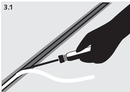
3.1 Remove filler using an appropriate tool, e.g. screwdriver.
