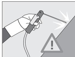
⚠️ Welding of galvanised steel components produces hazardous fumes. Appropriate precautions should be taken to ensure safe working conditions for those in the vicinity of the welding operation.
