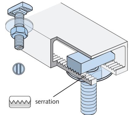
The notches on the T-bolt provide visual confirmation of T-bolt orientation; the final notch position must be at 90° to the channel's longitudinal axis.
