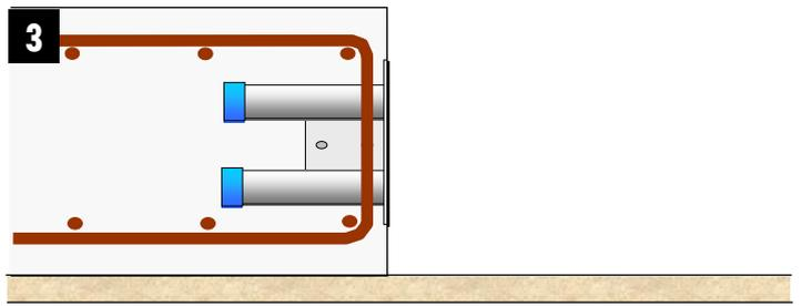
**3** When the concrete has achieved sufficient strength, strike shuttering and peel off or puncture the label
