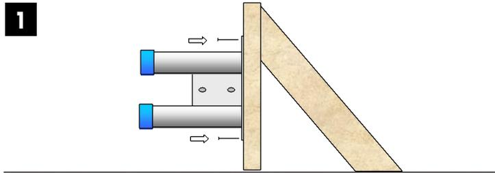
**1** Nail sleeve to formwork. Do not remove sticky label, this prevents ingress of concrete into the sleeve
