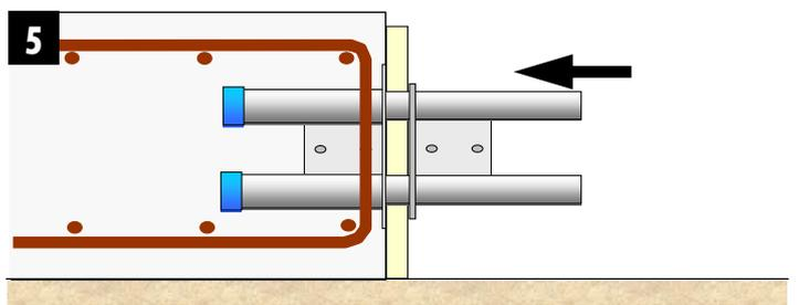
**5** Push the dowel component through the filler until it is fully located in the sleeve
