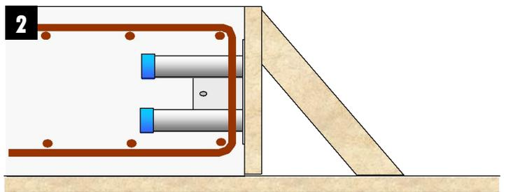
**2** Fix the local reinforcement around the sleeve and pour the concrete
