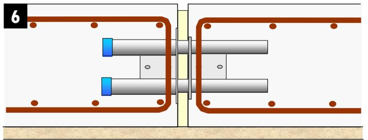
**6** Fix the local reinforcement around the sleeve and pour the concrete
