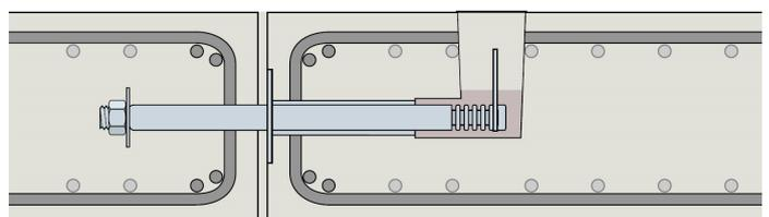
**Notes:** Where deep concrete pours are proposed, the installation will require further consideration. More robust fixing of the sleeve and dowel components will be necessary, to avoid displacement during casting of the concrete. Ensure joint has been filled before pouring resin.
