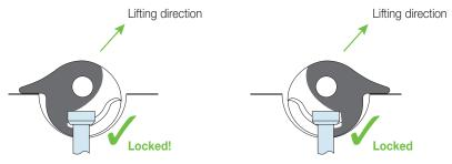
The locking well prevents sphere rotation and permits loading towards or away from the tail. This eliminates the risk for mis-connection, reduces wear and prevents lip distortion.
