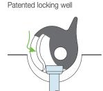
The lips of the slot slide around the anchor head which drops into the locking well.
