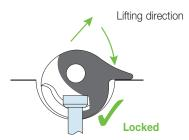
Supervision is required to ensure that the clutch is correctly connected for safe lifting toward the tail!
