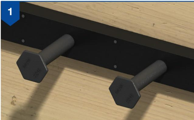
RT KSN Anchors are inserted into the Ancon RT KSN Anchor Block. The unit is then nailed to the formwork. The wall reinforcement is installed to which the anchors are tied. The concrete is cast and once it reaches sufficient strength, the formwork is removed.
