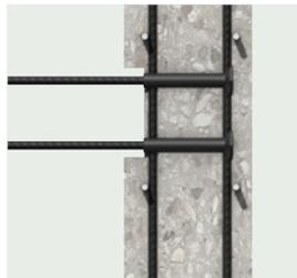
High performance RT KSN Anchor System. Bars are installed when required. No bending of bars. Less congestion in the wall.
