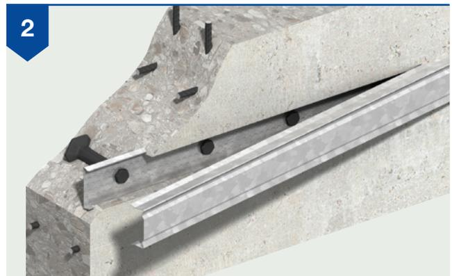
When a connection is required, the cover is removed and the bolts which held the Anchors to the casing prior to installation are removed to reveal the threads.
