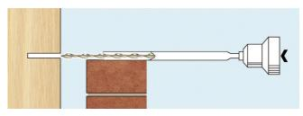
2. Load tie into support tool and line up with pilot hole while resting support tool on new leaf.
