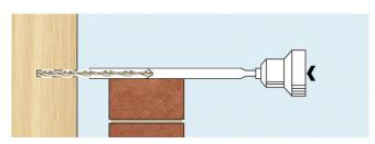
**3.** Drive in tie with SDS drill. (If insulation is installed, fit retaining clip over the StarTie).
