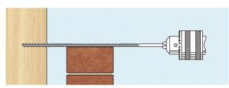
1. Drill pilot hole into existing wall (not required with low density timber).
