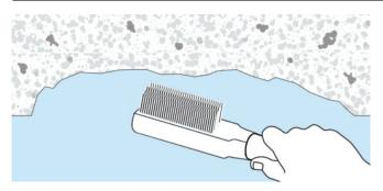
Remove all loose concrete from the area to be patched. Hammer tap the area to establish if any hollows are present and break back to sound concrete. Remove any dust and debris with a stiff wire brush. Clean and treat any exposed embedded steel rebar with a suitable epoxy coating.
