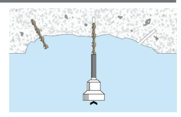
3. Fit the PatchPin support tool over the drill bit and insert the PatchPin into the tool. Install the PatchPin into the pilot hole with the SDS rotary hammer drill set to hammer only. Ensure that the outer end of the pin will be below the face of the concrete patch – the pin can be bent, if required.
