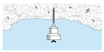
Drill pilot holes, vertically or at an angle of up to 45°, to the correct diameter and spacing into the concrete (using an SDS rotary hammer drill).
